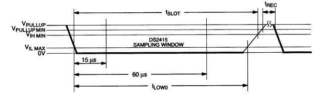
$60\mu s \leq t_{LOW0} < t_{SLOT} < 120\mu s \\ 1\mu s \leq t_{REC} < \infty$
